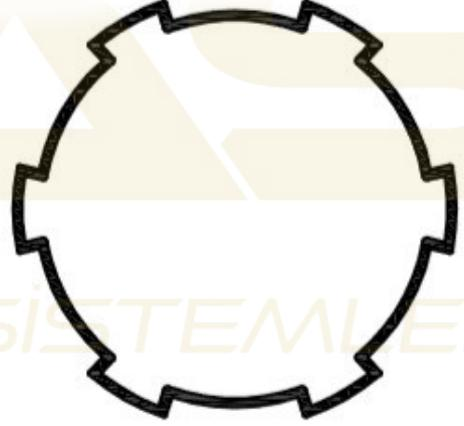
Motor Boru adaptör içten Profili / Internal Profile of Engine Pipe Adapter
